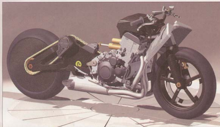
Where's the chassis? You're looking at it. The inline-Four engine's cases are structural and carry mounts for the swingarm and “double-wishbone” alternative front suspension.
